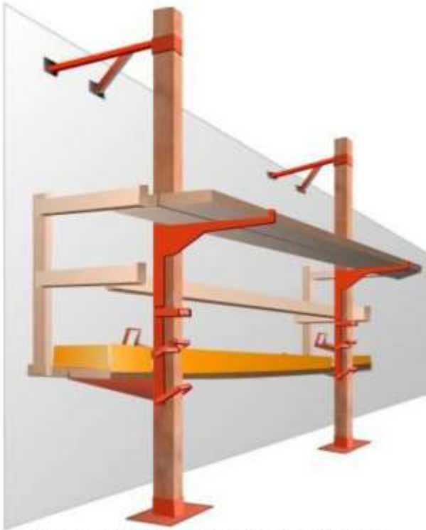
An example of Pump Jacks showing all features.
